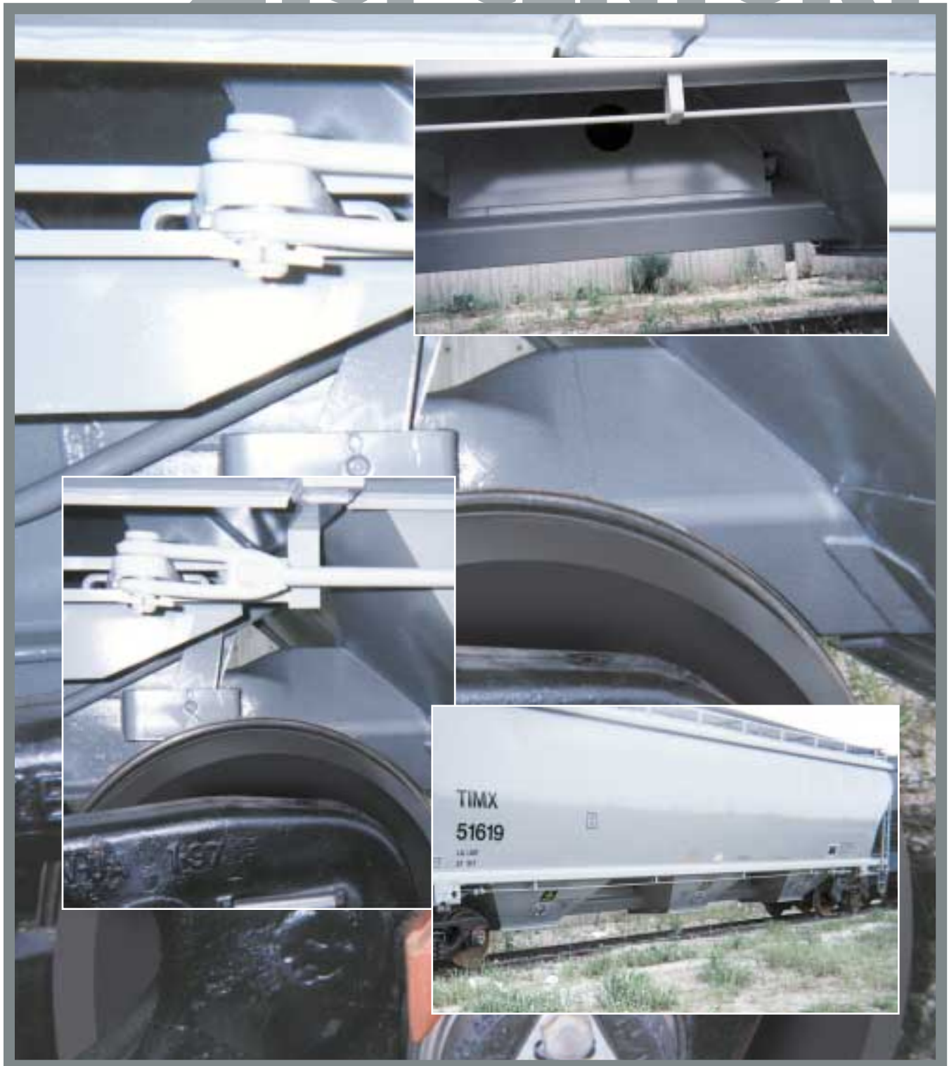
14" square HSS (located just above the wheel) provide the structural "spine" for railroad grain cars.
