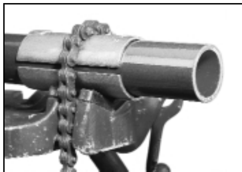
Figure 15: Field-fabricated half shell clamps used with chain vise to protect PVC-coated conduit. (Courtesy of ROBROY Industries Conduit Division)
