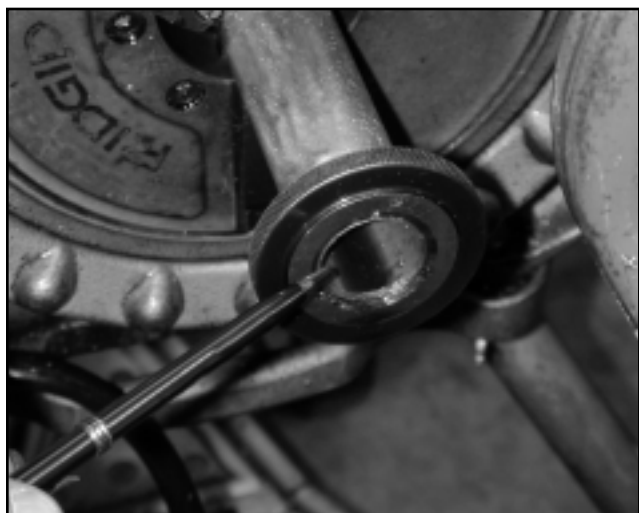
Figure 11: Threads should be checked with a NPT-L1 threaded ring gauge to ensure proper make up. (Courtesy of Wheatland Tube)
