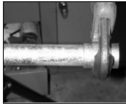
Figure 19: To avoid damaging the PVC coating, use an EMT shoe one trade size larger than the conduit being bent. (Courtesy of ROBROY Industries Conduit Division)
