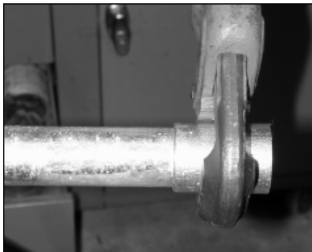
Figure 13: When assembled wrench-tight the coupling will cover all threads. (Courtesy of Wheatland Tube)
