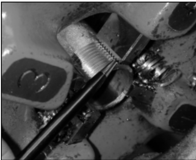
Figure 9: When proper thread length is achieved the end of the conduit becomes flush with the ends of the die segments. (Courtesy of Wheatland Tube)
