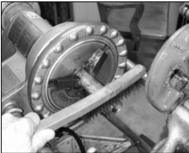
Figure 10: Wire brush the threads to remove any shavings or debris. (Courtesy of Wheatland Tube)
