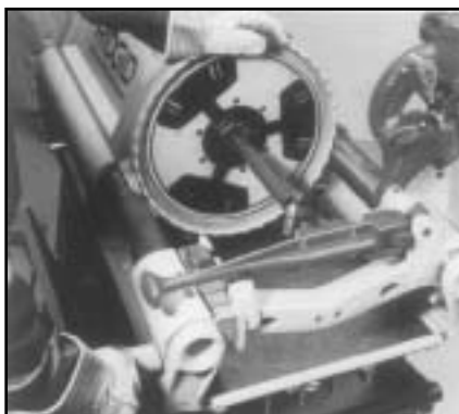
Figure 18: Using a reamer to remove rough edges of cut PVC-coated conduit. (Courtesy of ROBROY Industries Conduit Division)
